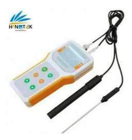
Jpb-607a portable intelligent dissolved oxygen analyzer (hereinafter referred to as the instrument) is mainly designed for the convenience of users to carry to the field operation. The instrument can be divided into two parts: sensor and electronic unit. The sensor adopts polarographic coated dissolved oxygen electrode. The electronic unit is composed of high integrated circuits. The instrument adopts the lattice liquid crystal display, which can show the dissolved oxygen value and temperature.
