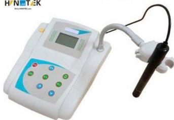
A dissolved oxygen meter measures the amount of oxygen dissolved in an aqueous solution. Oxygen is dissolved in water by surrounding air, air flow, and photosynthesis.
