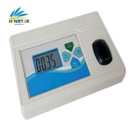
The wgz-xt bacterial turbidity meter is mainly used to measure the concentration of bacteria in the suspension of the strain to be identified. The instrument was calibrated with (BaSO4) McFarland standard solution and McFarland McFarland unit. The metric turbidity value is directly shown. It is suitable for the determination of bacteria and bacteria concentration in medical and health units, biological products, quarantine institutions and scientific research institutions.
