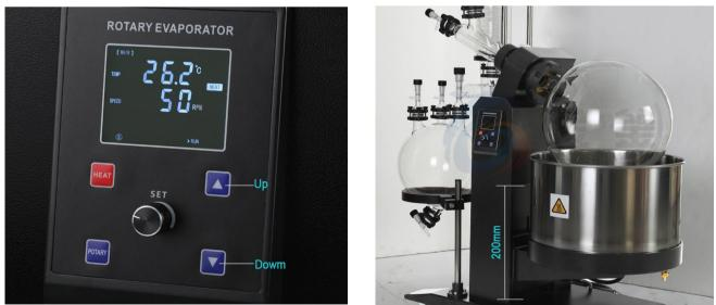
The temperature is controlled by "Super Fuzzy PID", with smaller temp. overshoot, faster stable time, better temp. control accuracy, "F and °C can be switched. RS485 communication is optional;
