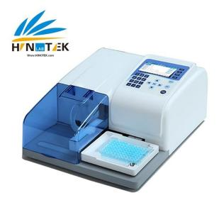
The APW-100 Microplate Washer is easy, convenient and versatile to use for washing microplate in ELISA assays. It efficiently removes liquid from wells. Low residual volumes eliminate high background signal to ensure reliable assay results. Washing performance can be optimized by adjusting wash parameters, such as wash cycles, soaking time, shaking speed, dispense and aspiration height and speed.
