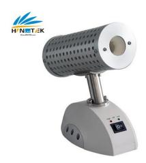
HM-3000A and HM-3000C Bacti-Cinerator Sterilizer sterilizes micro-organisms utilizing infrared heat produced by a ceramic core element. The ceramic element contains no asbestos and ensures maximum sterility without splatter across the work surface area. Complete sterilization occurs within 5-7 seconds at optimum sterilizing temperature of 1500°F (815.6°C).
