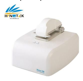
The Nano-100 is a perfect instrument for micro-volume UV-VIS spectrophotometer. It can accurately measure DNA, RNA and Oligonucleotide concentrations, protein assays etc. The Nano-100 utilizes CCD detector, a light source for long lifetime Xenon lamp, together with simple software. Simply pipette 0.5~2µl sample onto the pedestal, and the measurement can be completed within 5 seconds.
