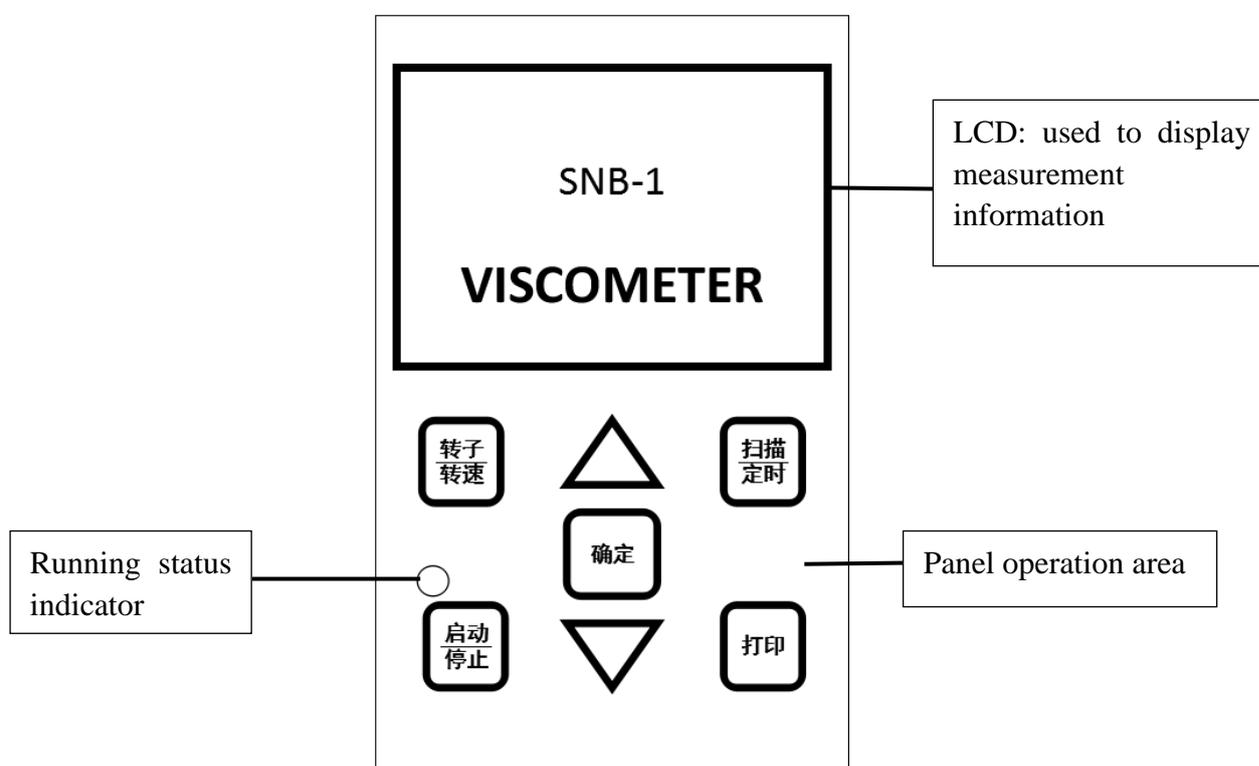
After the boot, the instrument first displays the instrument type information and waits for 3 seconds to get into the test state. At this point, there are 4 lines in the LCD screen:
