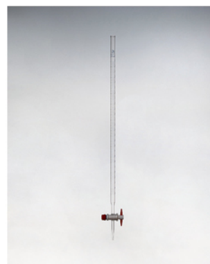
BURETTE Class A & Class B with blue line on milk white background, straight stopcock
