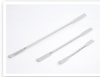
药刮 Spatulas Stainless steel AISI304. One end rounded and bends up, one end square
