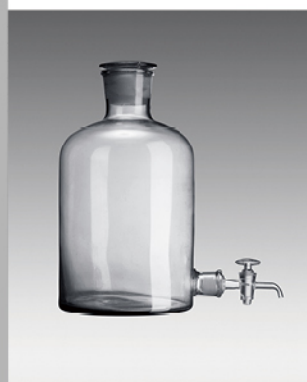
ASPIRATIR BOTTLE with ground-in glass stopper and stopcock at bottom SODA GLASS
