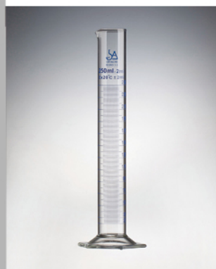
MEASURING CYLINDER hexagon with spout BORO 3.3
