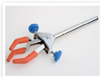
三爪双调节多用夹 Three Finger Double Adjust Clamp Double adjustable, PVC coated prongs. Made of chrome plated zinc-alloy. Accept objects from 0-30mm, 0-70mm
