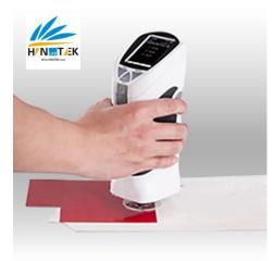
Spectral colorimeter is the colorimeter which adopts the theory of spectrophotometer. It is widely used for plastic, printing, paint, ink, textile, dyeing and other industries for color management. It could measure the target  $L^*a^*b$ ,  $L^*c^*h$  and the sample  $\Delta E$  and  $\Delta Lab$  value.
