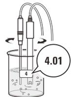
The meter will automatically recognize the buffer solution and begin the calibration, the Calibration icon continuously flashing.
