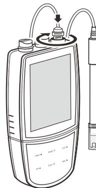
2. Remove the protective cap from the bottom of electrode. If tiny air bubbles are present inside the pH-sensitive glass membrane, gently shake the electrode downward to remove air bubbles.
