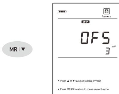
2.4 To exit the calibration log, press the **Meas** key.
