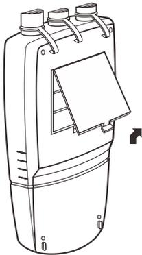
2. Insert three AA alkaline batteries into the battery compartment, note polarity.
