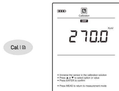
1.3 If necessary, press the **▲** / **▼** key to set the calibration value.
