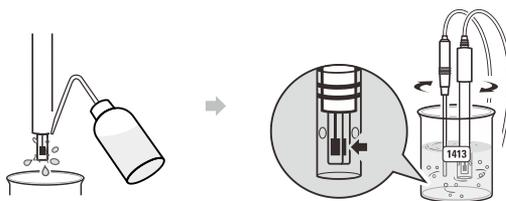
The meter will automatically show the calibration standard (e.g., 1413  $\mu\text{S}/\text{cm}$ ).
