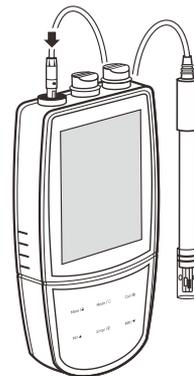
After connection is completed, DO NOT pull on the sensor cable. Always make sure that the connector is clean and dry.
