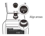
5. Press the **Enter** key, the meter begins calibration. The Calibrating icon shows on the upper right corner of the screen.
