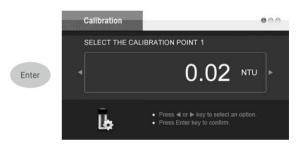
Take out the corresponding turbidity standard from accessory box (e.g., 0.02 NTU), wipe the vial with a lint-free cloth to remove fingerprints. Hold the vial cap and gently inverting vial several times, ensure that the turbidity standard is homogeneous and no air bubbles.
