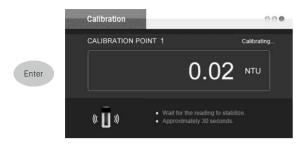
When the reading stabilizes, the meter will automatically show next calibration point.
