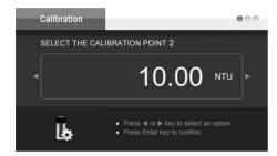
If necessary, press the ▶ key to select a desired calibration point.
