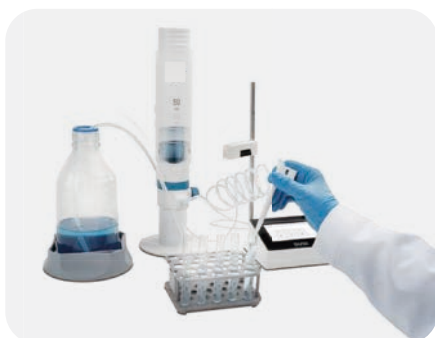
Automatic multi-step dispensing: Set dispensing volumes for different steps (step1, step2...step10, up to 10 steps, with total volume not exceeding piston capacity), plus interval time; manually trigger the first dispense, then the program runs according to the set intervals.
