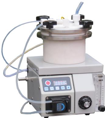
High precision peristaltic pump and atomizer
