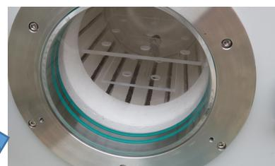
The large-diameter quartz vacuum chamber can process large-size thin-walled samples with uniform heating and good sintering effect.
