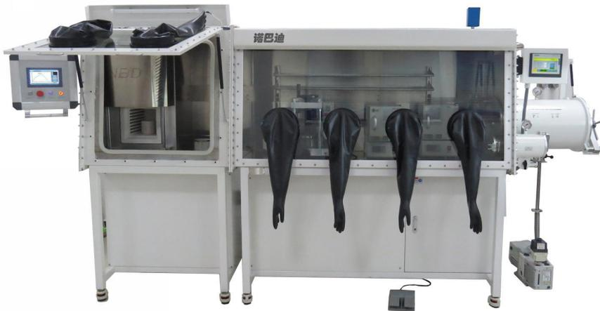
Glove box+High temperature sintering equipment
