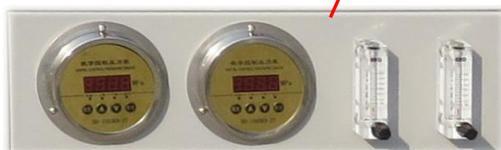
2-way pressure balance control and flow control systems
