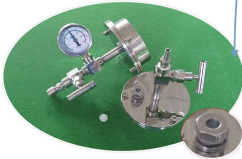
8mm Temperature Measuring hole in the flange
