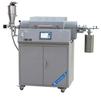
Continuous feed and discharge tilting atmosphere rotary furnace
