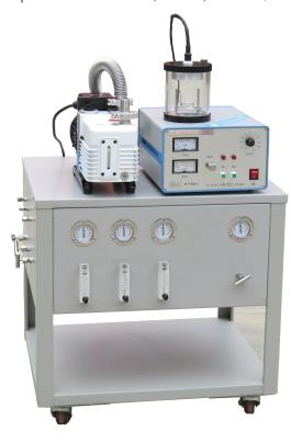
The far-source plasma sputtering system is different from the RF magnetron sputtering system in that sputtering is performed by generating a high-density plasma far from the target. Compared with conventional magnetron sputtering, the phenomenon of target poisoning is reduced, and the deposition rate of non-metal films is increased. At the same time can be applied to the target DC bias for sputtering insulating targets.
