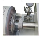
Measuring mechanism (vacuum degree: ≤ 5pa, mechanical pump)
