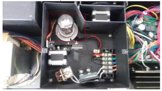
3. Pls. kindly check the voltage between the two positions. The normal value should be around 72V. If you could get that voltage, then we judge the lamp is broken and you need a spare part for replace.
